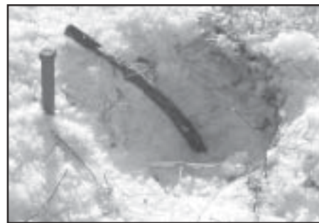
Facing southerly showing two posts; practitioner's is straight, original is bent. Plan states "Fd.I. Disturbed Re-est Pl. I. R1." New post not marked R1.
