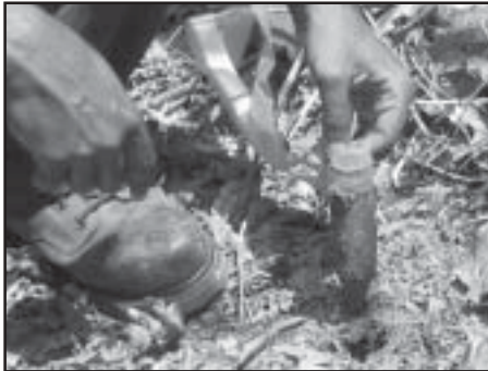
The lack of soil depth here on this sloping terrain necessitates using painted "bush pegs" for traverse points, as the local surveyor has done.
